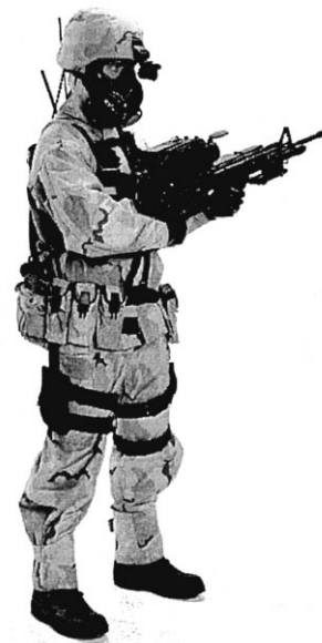
Fig. 2. Prototype land warrior system with AN/PAS-13 thermal weapon sight.
